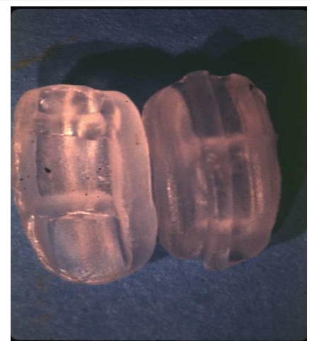
Figure 5. Enhanced Nitrification Bead shaped to protect biofilms during backwashing.
