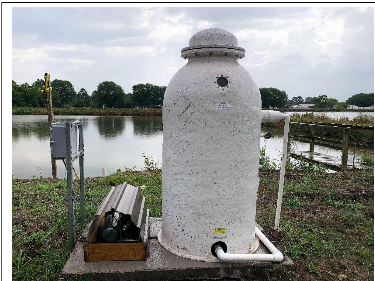
Figure 9. This HPPG 10 was positioned next to a lagoon where its ability to filter fine suspended solids is being tested on algal cells.
