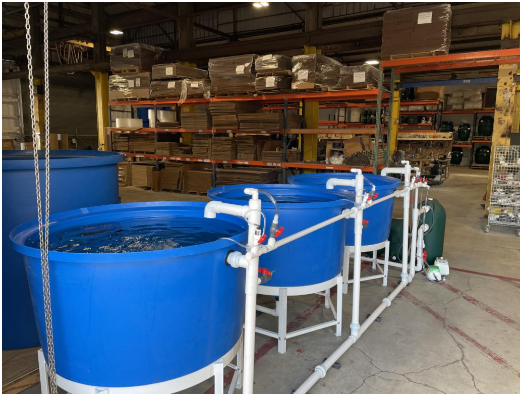
Figure 4. A special order MDC-3000 configured with cone bottom tanks under hydraulic testing. Three airlifts return water to the tanks powered by the larger linear air pump (upper right).
