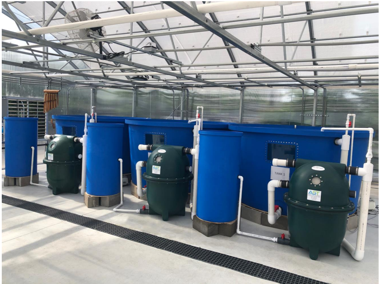
Figure 6. Three MDC systems assembled with a PG6000, 1200-gallon tank, and 3-inch airlift are supporting marine shrimp ( L. vannamei ) at a density of 10 kg/m 3 .
