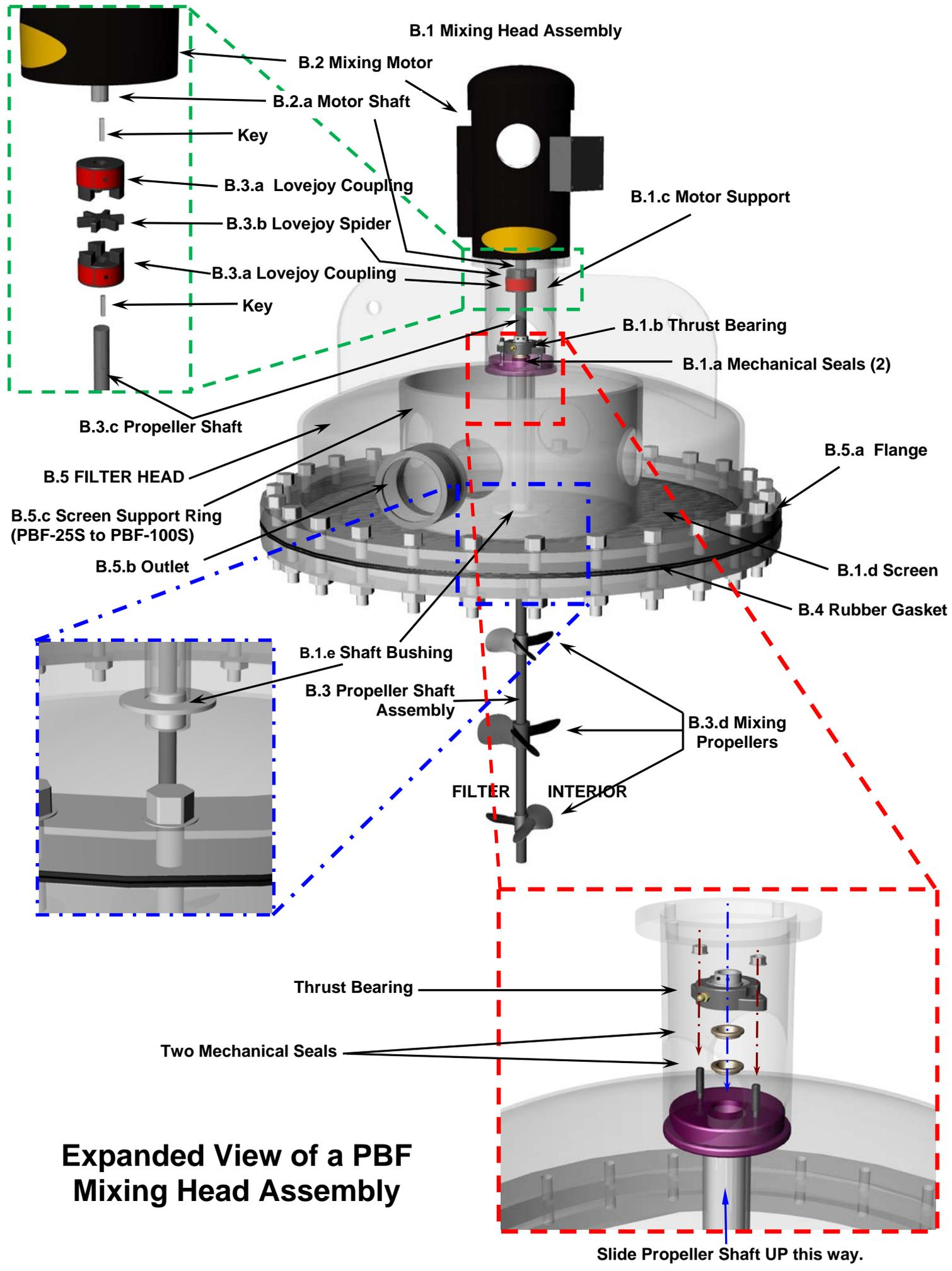
**Expanded View of a PBF Mixing Head Assembly**
