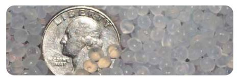
Bubble Bead filters backwash with a simple process. Turning off the pump and turning a few valves washes the dirty water and waste from the filter. After draining the dirty water, the pump is turned back on, the valves returned to their starting position, and the system resumes normal filtration. The bead media (*pictured above*) captures physical waste and debris, and never needs to be replaced.
