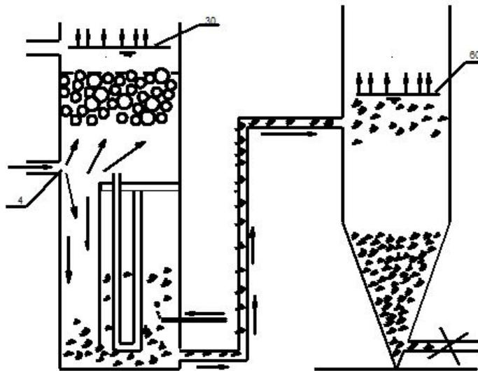
It is important to drain the open sludge reservoir periodically as a buildup of nitrites and nitrates will occur as the wastes breakdown. A consistent water level will be maintained in the culture system even as solids are being sent into the sludge reservoir
