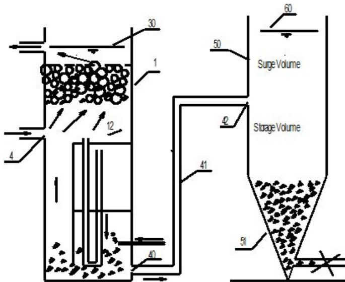
The PolyGeyser® filter in the FIT systems, also includes a built in sludge reservoir. When the trigger fires, clarified water on the top of the external reservoir is drawn back into the system. At the end of the backwash, the sludge from the filter is forced through the connecting pipe into the external reservoir. There, the sludge settles to the bottom and clarified water inhabits the upper level of the reservoir. The clarified water is where the exchange water is pulled from.
